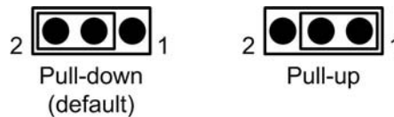
Figure 7. W1 jumper configurations
