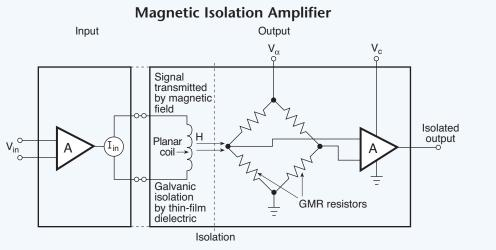
Fig. 5.24A. Magnetic couplers transfer signals through a magnetic field across a thin film dielectric. In this case, a magneto-resistance bridge circuit sensitive to the field exhibits a large change in resistance when exposed to the magnetic field from a small coil sitting above it.
