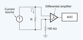
Fig. 4.06. Sensors with 4 to 20 mA outputs are typically placed in series with a resistor to develop a voltage. The resistor is then connected to the input of a differential amplifier to measure the voltage drop.
