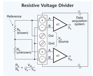
Fig. 4.10. Resistive voltage dividers work with single-ended or differential amplifiers and a reference resistor whose value is near the unknown resistor's value.
