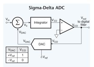
Fig. 2.04. Integrating converters such as the sigmadelta ADC have both high resolution and exceptional noise rejection. They work particularly well for low-bandwidth measurements and reject high-frequency noise as well as 50/60 Hz interference.
