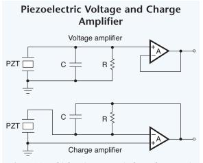
Fig. 8.03. A high-gain op amp isolates the sensor's output voltage from the effect of signal cable capacitance and lets the amplifier reside several meters away from the sensor.
