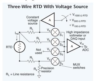
**Fig. 6.16.** This is a variation of the four-wire circuit with a voltage source and a stable sense resistor.
