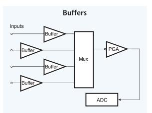
Fig. 3.04. Buffering signals ahead of the multiplexer increases accuracy, especially with high-impedance sources or fast multiplexers
