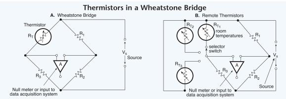
Fig. 6.24. An accurate temperature sensor can be fashioned from a thermistor in one leg of a bridge circuit. Lead length is not significant; so several sensors may be switched in and out of a single monitor without losing accuracy. Two thermistors make a differential thermometer that can be used for measuring temperature changes along a piping system or between various elevations in a building to balance the heating and air conditioning unit.
