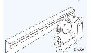
Rack and Pinion Encoder Assembly
