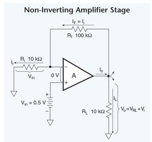
Fig. 5.06. The input and output polarities of the non-inverting amplifier are the same. The gain of the stage is  $A_{cl} = 11$  or  $(R_f + R_i)/R_i$ .
