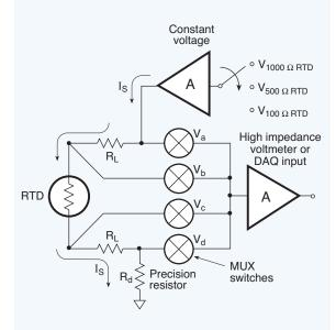
**Fig. 6.19.** Four voltage readings are taken for each RTD channel. The precision resistor measures  $I_s$ , the RTD current;  $V_b$  and  $V_c$  measure the RTD voltage; and the RTD resistance equals  $(V_b - V_c)/I_s$ .
