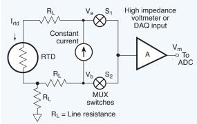
Fig. 6.14. The three-wire RTD method with a current supply is similar to the four-wire method. It simply eliminates one additional wire. Measure  $V_{\rm a}$  first, then measure  $V_{\rm b}$ .
