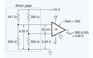
Fig. 7.06. Normally, the strain gage signal in a Wheatstone bridge is superimposed on a commonmode voltage equal to half the excitation voltage. Consequently, a high CMRR is necessary to reject the common-mode voltage and amplify the strain gage signal.
