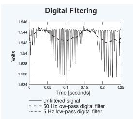
Fig. 3.15. The solid line is the noisy, unfiltered signal, and the two dashed lines show the same signal at the output of the 5 and 50 Hz low-pass digital filters.
