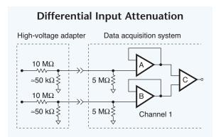
**Fig. 4.02.** A differential amplifier requires a resistor at both inputs when running single-ended, but only one resistor in a voltage-divider attenuator.
