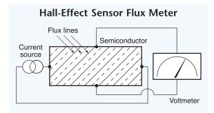
Fig. 4.08. When either the voltage or current port is regulated and calibrated, the Hall-effect device can be used as a magnetic flux sensor. The unregulated port provides an output signal proportional to the magnitude of unknown flux density. However, a Hall-effect proximity sensor or switch is a more widely used component based on this principle.
