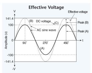
**Fig. 4.03.** The numerical value for the peak voltage of ac must be 1.414 times that of dc to produce the same heating effect.
