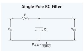
Fig. 10.14. Passive single pole filters are moderately effective in passing a band of frequencies that contain the measured signal, while attenuating other frequencies containing noise.
