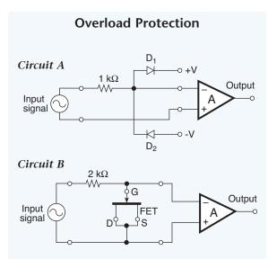
Fig. 5.35. Certain CMOS multiplexers may be protected against overvoltage destruction with diode and resistor networks that shut down any parasitic transistors in the device, limit the current input to a safe level, and shunt input signals to ground when the power supplies are turned off (Circuit A). JFET transistors also protect multiplexer inputs when they are connected as diodes. The JFET clamps at about 0.6 V, protecting the sensitive op amp input from destruction (Circuit B).
