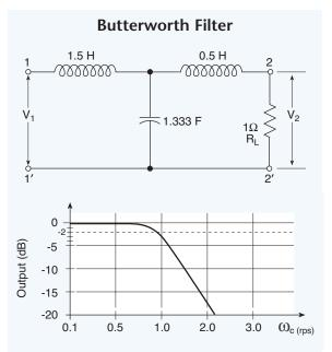
Fig. 5.12A. Butterworth filter and response characteristics
