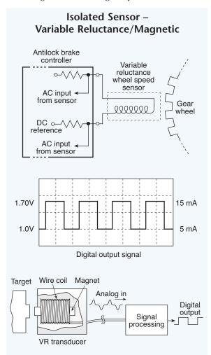
Fig. 5.28. Variable reluctance sensors comprise a coil of wire wound around a magnetic core. As a ferrous metal passes near one pole it disturbs the magnetic field and induces a small voltage in the coil. In this example, the voltage is amplified, shaped, and converted to a digital signal for indicating vehicle wheel speed.
