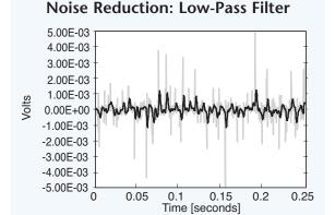
Fig. 10.16. An active, three-pole low-pass filter, configured as a Butterworth, Bessel, or Chebyshev filter, reduces the noise signal more effectively without significant attenuation than does a passive circuit.
