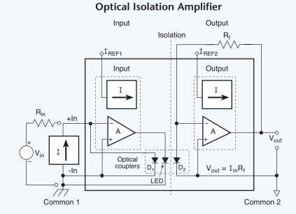
**Fig. 5.23.** This is a simplified diagram of a unity gain current amplifier using optical couplers between input and output stages to achieve isolation. The output current passing through the feedback resistor (R<sub>f</sub>) generates the output voltage.
