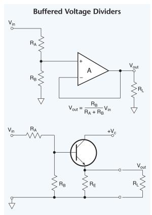
Fig. 5.18. An op amp or a transistor serves as an impedance matching buffer to prevent the load from affecting the divider's output voltage.
