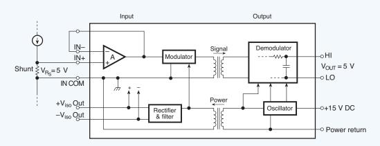
Fig. 10.08. This instrumentation amplifier with transformer coupling is typically used in an industrial process control loop and provides galvanic isolation in both input and output circuits. It can measure a  $\pm 5$  Vdc signal riding on a common-mode voltage as high as 2000 V.
