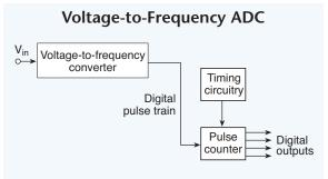
Fig. 2.02. Voltage-to-frequency converters reject noise well and frequently are used for measuring slow signals or those in noisy environments.
