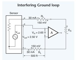
Fig. 10.03. The 150 mV dropped across  $R_L$  in the bottom ground return line arises from the 30 mA of current flowing in 5.2  $\Omega$  of lead wire resistance. The voltage adds to the sensor's 2.50-V signal to yield 2.65 V at the input to the signal-conditioning amplifier and produces a 6.6% error.
