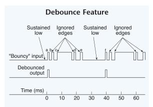
Fig. 11.07. A relay contact debounce circuit filters extraneous signals that the measurement amplifier could mistake for rising and falling edges of a legitimate string of signal pulses.
