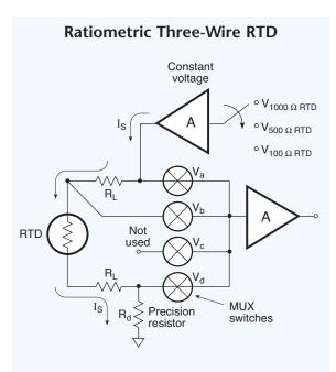
Fig. 6.20. The three-wire ratiometric circuit assumes that both sense-wire resistances in the four-wire circuit are the same. The equation for calculating RTD resistance simply accounts for it with a factor of two.
