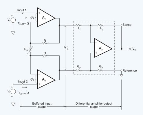
Fig. 5.11. The instrumentation amplifier exhibits extremely high impedance to the inputs  $V_1$  and  $V_2$ . Resistor  $R_m$  adjusts the gain, and the single-ended output is a function of the difference between  $V_1$  and  $V_2$ .
