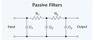
**Fig. 6.08A.** Passive filters come in a variety of configurations to suit the application. They are built in single or multiple sections to provide increasingly steeper slopes for faster roll-off.
