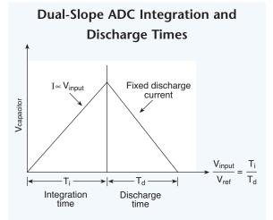
Fig. 2.03. Dual-slope integrating ADCs provide high-resolution measurements with excellent noise rejection. They integrate upward from an unknown voltage and then integrate downward with a known source voltage. They are more accurate than single slope ADCs because component errors are washed out during the de-integration period.
