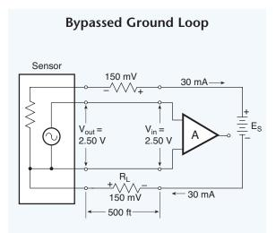
Fig. 10.04. A separate wire run from the sensor ground (or common terminal) bypasses the power supply ground wire voltage drop. The true output signal of the sensor (Vout) reaches the amplifier input terminals because the input draws negligible current.
