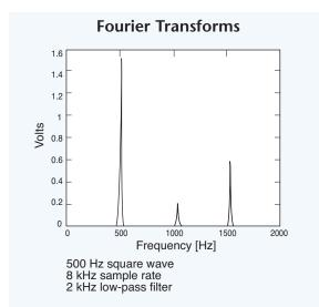
**Fig. 3.10.** The Fourier Transform of a 500 Hz square wave is sampled at 8 kHz with a low-pass filter cutoff at 2 kHz.
