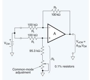
Fig. 10.07. Common-mode voltage is measured between the two input terminals and the common terminal. Because the two inputs must have identical voltages, they may be tied together and connected to one voltage source.
