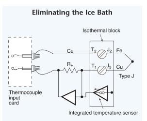
Fig. 6.06. A thermistor sensor placed near the lead wire connections is an alternative method of replacing the ice bath. The measured temperature is the difference between the thermocouple temperature and the reference thermistor temperature.
