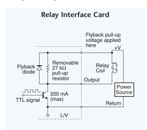
**Fig. 11.02.** A plug-in card containing a special digital amplifier is often provided to interface a TTL signal to a control relay. The amplifier can boost the standard 5 V TTL signal to 24 Vdc at 200 mA.
