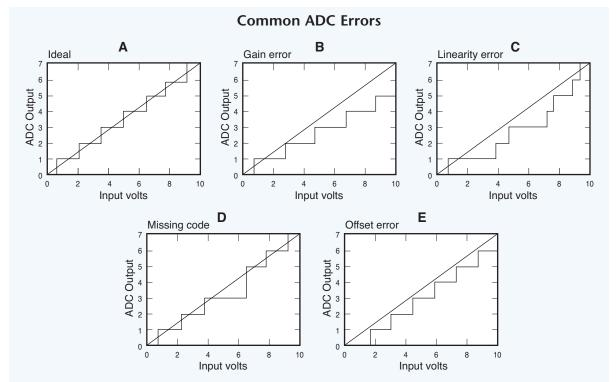
**Fig. 2.07.** The straight line in each graph represents the analog input voltage and the perfect output voltage reading from an ADC with infinite resolution. The step function in Graph A shows the ideal response for a 3-bit ADC. Graphs B, C, D, and E show the effect on ADC output from the various identified errors.
