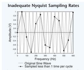
**Fig. 3.06.** When sampling an ac signal at less than two times the Nyquist frequency, the original waveform cannot be reproduced faithfully.
