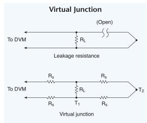
Fig. 6.09. A short circuit or an insulation failure between the leads of a thermocouple can form an unwanted, inadvertent thermocouple junction called a virtual junction.
