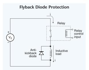
Fig. 11.01. The fly-back diode clips high voltage spikes ordinarily developed across the inductive load when the control relay contacts open. Without diodes, the high voltage arcs across the opening contacts, substantially reducing their useful life.
