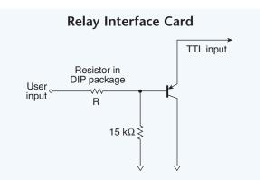
Fig. 11.03. One optional interface card comes with an adjustable attenuator to handle an input range from 5 to 48 V in four steps. The table specifies the voltage levels that can be selected with four different resistors.
