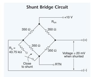
**Fig. 7.07.** A bridge may be calibrated with a shunt resistor, which is switched with a software command into either one of the two lower legs.
