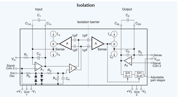
**Fig. 5.20.** A differential isolation amplifier's front end can float as high as the value of the common mode voltage (CMV) rating without damage or diminished accuracy. The isolation barrier in some signal conditioners can withstand from 1,500 to 2,200 Vdc.
