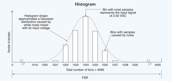
Fig. 2.08. The histogram illustrates how 12-bit ADC samples in a set were distributed among the various codes for a 2.5 V measurement in a FSR (full-scale range) of 10 V. Most codes intended for the 1024 bin representing 2.5 V actually ended up there, but others fell under a gaussian distribution due to white noise content.
