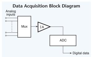
Fig. 5.01. A simple data acquisition system is composed of a multiplexed input stage, followed by an instrumentation amplifier that feeds one accurate and relatively expensive ADC. This arrangement saves the cost of multiple ADCs.
