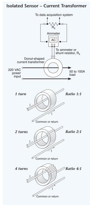
**Fig. 5.27.** Because it does not need a ground connection, a current transformer is isolated from both the input and output of the signal conditioner.
