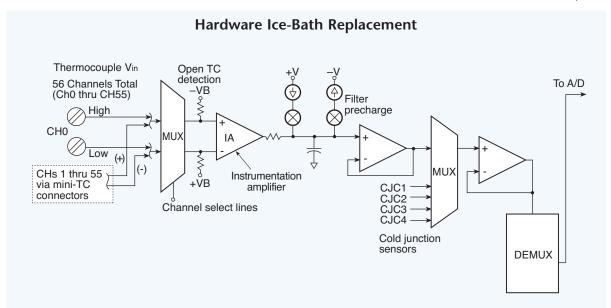
**Fig. 6.07B.** A typical input scanning module can accommodate up to 56 thermocouples of any type, and up to 896 channels can be connected to one analog-to-digital mainframe.
