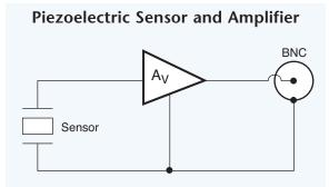
Fig. 8.04. Some piezoelectric accelerometers come with built-in amplifiers. They have a low output impedance and require an external power supply.
