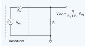
Fig. 5.03A. The sensor's source impedance  $R_S$  should be relatively small to increase the voltage divider drop across  $R_i$ , the amplifier's input. This can substantially improve the signal-to-noise ratio for mV range sensor signals.
