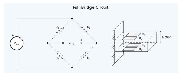
Fig. 7.01. The full-bridge circuit provides the largest output with minimum errors. All four arms of the bridge are active; two are in tension while the two on the opposite side are in compression.
