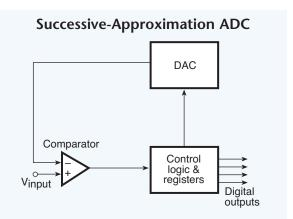
Fig. 2.01. Interestingly, this ADC uses a digital-toanalog converter and a comparator. The logic sets the DAC to zero and starts counting up, setting each following bit until it reaches the value of the measured input voltage. The conversion is then finished and the final number is stored in the register.
