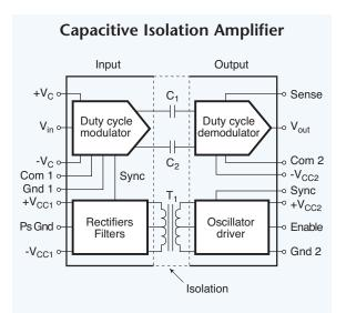
Fig. 5.22. The isolation barrier in this amplifier protects both the signal path and the power supply from CMV breakdown. The signal couples through a capacitor and the power through an isolation transformer.
