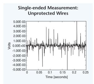
Fig. 10.05. Radiated noise spikes are easily picked up on non-twisted, non-parallel, unshielded lead wires connected to the single-ended amplifier input terminals, even when the inputs are shorted together.
