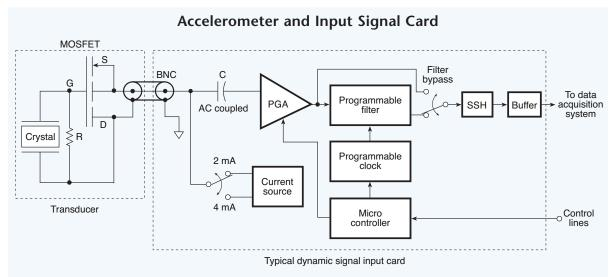
Fig. 8.05. A piezoelectric accelerometer with a built-in MOSFET amplifier stage drives a programmable gain amplifier on a dynamic signal input card. The 2 or 4 mA current source powers the MOSFET.
