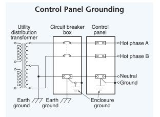
**Fig. 10.01.** Utility power transformers are typically grounded to earth ground near the transformer, and again at the input to the electrical junction box or first switching panel. The switching panel, in turn, may be connected to a rod driven into the earth to ensure that it too is at true ground potential.
