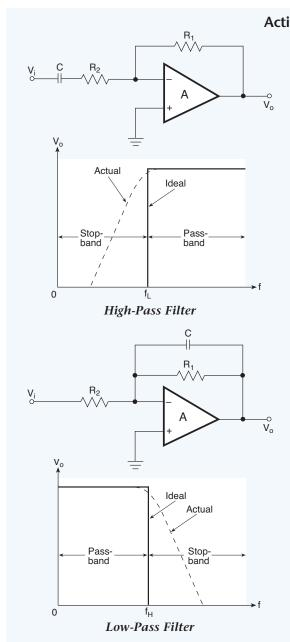
Fig. 5.15. Passive filters tend to change in frequency-cutoff characteristics with a change in load. To prevent this, an active device such as a transistor or op amp isolates the last pole from the load to maintain stable filter characteristics.
