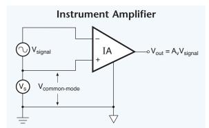
Fig. 5.09. An instrumentation amplifier is typically a differential input operational amplifier with a high common-mode rejection ratio.
