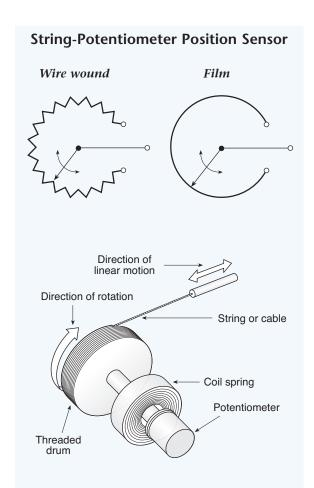
Fig. 9.01. String potentiometers occupy relatively little overall space in a machine installation or device under test. In some applications where a sensor cannot be mounted on the device being measured, the potentiometer may be conveniently located some distance from the test bed without sacrificing accuracy or repeatability.
