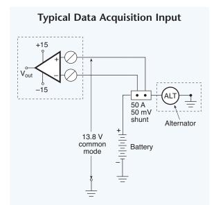
Fig. 4.04. The battery charging current in an automobile electrical system is typically measured with a handheld diagnostic voltmeter across a shunt resistor, which is totally isolated from the battery voltage. However, when a data acquisition input amplifier is connected to the shunt, the input also must sustain the common mode voltage represented by the battery.
