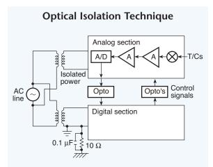
Fig. 10.09. Optical devices are the most widely used component for coupling signals across high-potential barriers and for low-level signals that are prone to the electrical noise typically coupled through different ground potentials.
