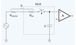
Fig. 5.02. The source resistance should be as low as possible to minimize the time constant of the MUX's parasitic capacitance C and series resistance R. An excessively long time constant can adversely affect the circuit's measurement accuracy.
