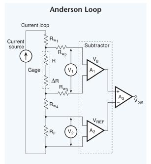
Fig. 4.12. The Anderson loop uses a unique subtractor circuit, which eliminates errors arising from lead wire resistance. It measures only the sensing element's resistance change.
