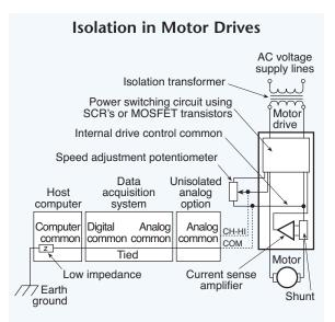
Fig. 10.12. Common-mode voltage is defined as the voltage between a signal and the localized common, which is usually earth ground. Common-mode voltages can be quite high, depending on the signal source. For example, a current sensing shunt in a dc motor drive might be expected to be at line-voltage potential, although the actual signal level is less than 50 mV across the shunt terminals. Measurement techniques for small signals at high common mode potentials call for isolation.
