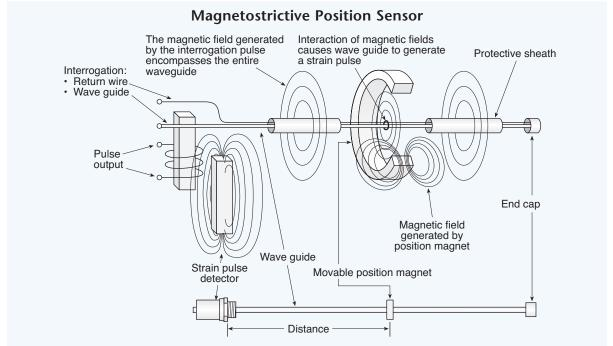
**Fig. 9.03.** Magnetostrictive position sensors have a high signal-to-noise ratio, shock and vibration resistance, and accuracy. They are rugged devices that deliver from 30 to 400 mV signals at their output terminals and require little or no additional signal conditioning. A possible disadvantage for some applications, however, is its wave-guide, which must be at least as long as the measured stroke.
