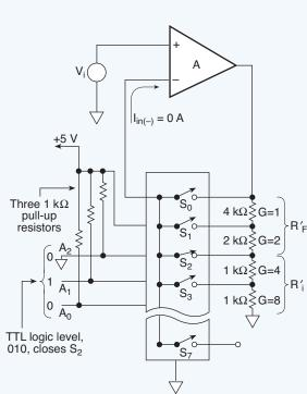
Fig. 5.08. The non-inverting amplifier is configured for programmable gain and controlled by the binary input signals from a computer to the addressable inputs of the analog switch.
