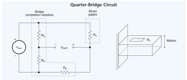
Fig. 7.03. A quarter-bridge circuit uses only one active arm and is the least sensitive of the three types. It is also the most prone to noise and errors.
