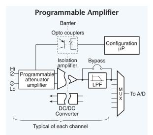
Fig. 10.11 All three techniques of isolation are used in a multi-channel, programmable amplifier. Optical devices couple digital signals, capacitors couple analog signals, and the dc/dc converter supplies power to the isolated side.
