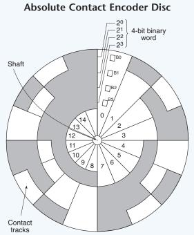
**Fig. 9.06.** The disc pattern on the contacting encoder is a digital word, which represents the absolute position of the encoder shaft.
