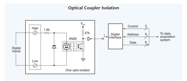
Fig. 11.05. An optical isolator decouples the digital signal source ground from the data acquisition system ground, and protects the acquisition system inputs from unintentional high voltages.
