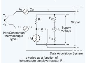
Fig. 6.07A. A number of electronic circuits or modules can replace the ice-bath. The temperature-sensitive resistor changes the calibrated value of voltage e in proportion to the amount of temperature compensation required.
