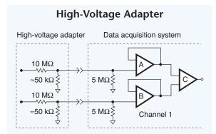
Fig. 4.01. A typical data acquisition system usually requires an attenuator at its input to accept voltages that exceed 10 V.
