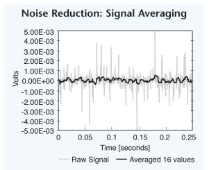
Fig. 10.13. Signal-averaging using software techniques virtually reduce the effective electrical noise pick up before the data acquisition system processes the measured signal.
