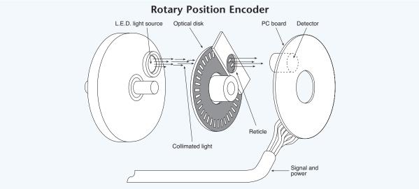
**Fig. 9.07.** The shutter is one of the most critical components of the encoder assembly. The sensor's resolution and accuracy hinge on the quality of the vendor's manufacturing and assembly processes.
