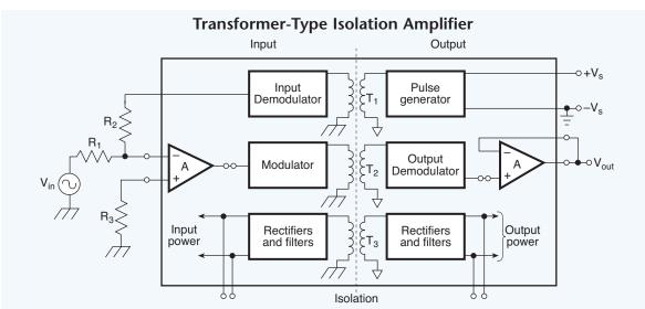
**Fig. 5.24B.** The transformer-coupled isolation amplifier uses separate power supplies for the input and output stages, which are isolated by virtue of the individual transformer windings. This provides the input and output stages with decoupled ground or common returns. In addition, the modulator/demodulator transfers the measured signal across the barrier via other transformer windings for complete galvanic isolation between input and output.
