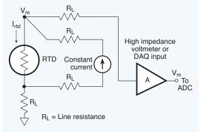
**Fig. 6.13.** The four-wire RTD method with a current supply eliminates the lead wire resistance as a source of error.
