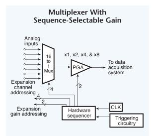
Fig. 3.03. A multiplexer with sequence-selectable gain lets the data system operate at its maximum acquisition rate.
