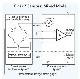
Fig. 12.03. Class 2 sensors use multiple leads to connect between the sensor and STIM. In the case of a Wheatstone Bridge circuit, for example, four leads connect the sensor and the other pair connects to the onboard TEDS EEPROM, which illustrates the mixed-mode application.
