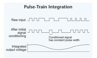
Fig. 11.08. In one type of frequency-to-voltage converter, an integrator circuit converts a string of constant-width pulses of varying repetition rate into a smoothly changing analog voltage. The analog signal is proportional to the input frequency.
