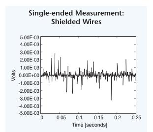
**Fig. 10.06.** Shielded wires reduce electrical noise pick up at the input of single-ended amplifier input terminals, but other techniques often are more effective.
