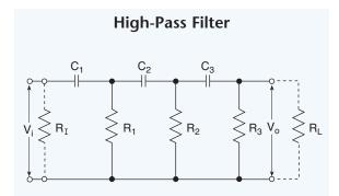
Fig. 5.14. The high-pass filter is designed to have a lower corner frequency near zero and the cutoff frequency at some higher value. The number of capacitor/resistor pairs determines the number of poles and the degree of cutoff sharpness.
