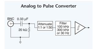
Fig. 11.06. An interface circuit contains an RC network that significantly attenuates ac signals below 25 Hz before converting the higher frequencies to a digital pulse stream.
