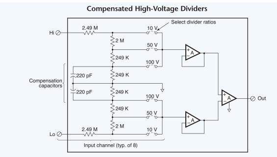
**Fig. 5.19.** A typical high-voltage input card for a data acquisition system contains a balanced differential input and jumpers for selecting an input voltage range of 10 V, 50 V, or 100 V. The input circuit also compensates for long lead wire capacitance that tends to form an ac voltage divider, which would reduce accuracy.
