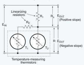
Fig. 6.22. The compensating resistors in series with the thermistors improve linearity near the center of the thermistor's S-shaped characteristic curve. This is where the sensitivity is the greatest, and its operating temperatures can be extended to cover a wider range.
