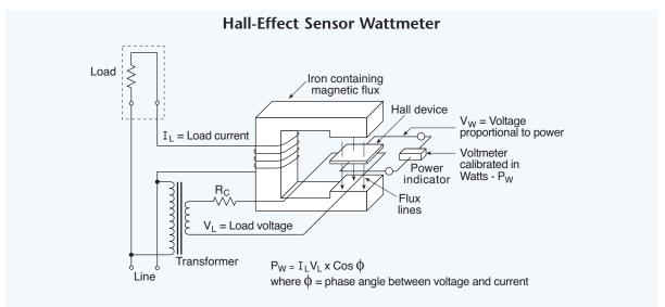
**Fig. 4.09.** A Hall-Effect sensor is an ideal wattmeter for measuring ac power. It inherently includes the phase angle between the voltage and current vectors as a multiplying factor to convert VA to W.
