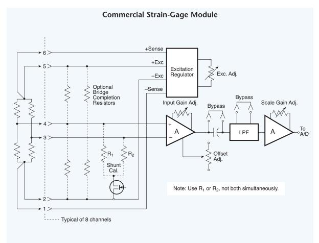
**Fig. 7.05.** A commercial strain gage module provides adjustable excitation, gain, and offset for each channel. This lets it make use of the instrument's entire dynamic range.
