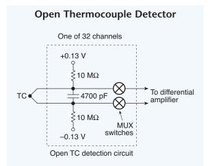
Fig. 6.11. The thermocouple provides a short-circuit path for dc around the capacitor, preventing it from charging through the resistors. When the thermocouple opens, due to rough handling or vibration, the capacitor charges and drives the input amplifier to the power supply rails, signaling a failure.
