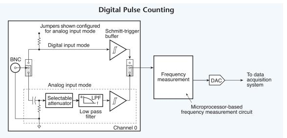
**Fig. 11.10.** In the other type of frequency-to-voltage converter, the input card contains an input coupling capacitor to filter low frequencies, an attenuator, a low pass filter, and a microprocessor to calculate the frequency. The signal is then connected to a DAC before feeding into the data acquisition system.
