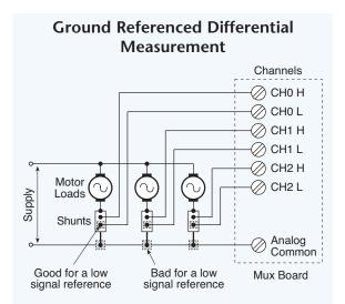
Fig. 4.05. High dc currents are often measured with shunts using differential inputs sharing a common ground.
