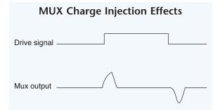
Fig. 5.03B. Analog-switching devices can produce spikes in the MUX output during level transitions in the drive signal. This is called charge-injection effect and can be minimized with low source impedance.
