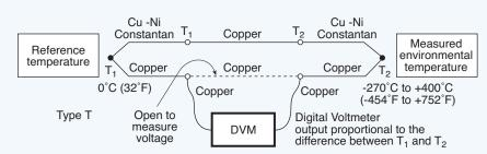
Fig. 6.01. A basic thermocouple measurement system requires two sensors, one for the environment under measurement and the other, a reference junction, normally held to  $0^{\circ}$ C ( $32^{\circ}$ F). Type-T is one of the dozen or more common thermocouples frequently used in general-purpose temperature measuring applications. It is made of copper and constantan metals and typically operates from -270 to  $+400^{\circ}$ C or -454 to  $+752^{\circ}$ F.
