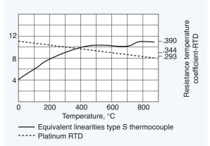
Fig. 6.17. Platinum is the material of choice for RTDs and thermocouples because it is stable and resists corrosion. Here, the RTD is shown to be more linear under temperatures of 800°C than the thermocouple.
