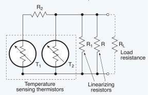
Fig. 6.23. Compensating resistors in the network linearize the resistance change vs. temperature in the same manner as they do for the voltage mode.
