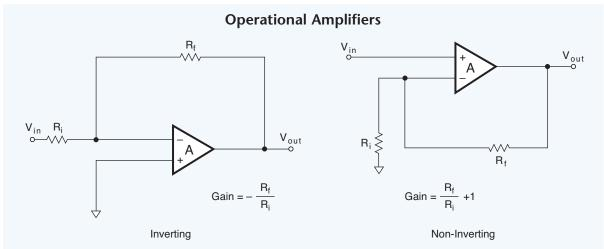
**Fig. 5.04.** The two basic types of operational amplifiers are called inverting and non-inverting. The stage gain equals the ratio between the feedback and input resistor values.
