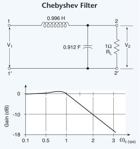
Fig. 5.12B. Chebyshev filter and response characteristics
