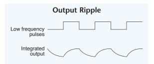
**Fig. 11.09.** The pulse-train integrator handles only frequencies above a certain cutoff, due to the integrator's time constant. Frequencies below cutoff produce output ripple if allowed to pass.
