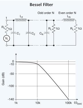
Fig. 5.12C. Bessel filter and response characteristics
