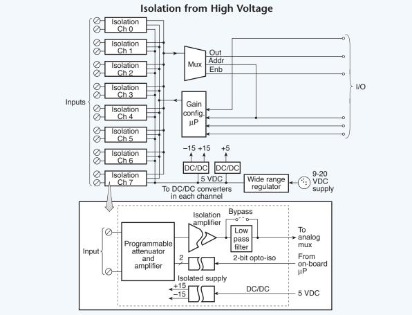
Fig. 5.34. The isolated voltage-input modules let data acquisition systems isolate several channels of analog input, up to 500 V channel-to-channel and channel-to-system.
