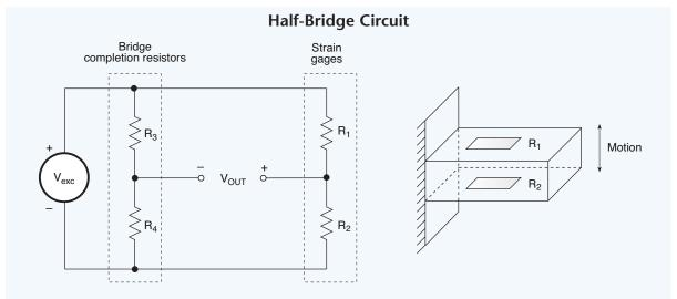
**Fig. 7.02.** In a half-bridge circuit, only two arms are active. Two strain gages are on the specimen while the two fixed resistors that complete the bridge are not.
