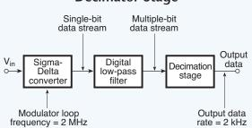
Fig. 2.05. Sigma-delta ADCs are well suited to highresolution acquisition because they use oversampling and often combine an analog modulator, a digital filter, and a decimator stage. The low-pass digital filter converts the analog modulator output to a digital signal for processing by the decimator.
