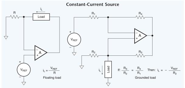
**Fig. 8.06.** A constant current source provides a source-gate bias for the field-effect transistor in the accelerometer. Depending on the specific FET circuit, a constant-current source may be configured for either a floating load or a grounded load.
