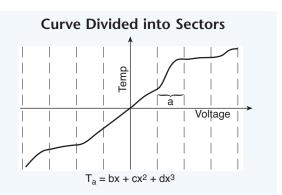
**Fig. 5.33.** Although a computer usually finds the solution to the NIST polynomial, breaking the curve into sections representing lower order polynomials can accelerate the process.
