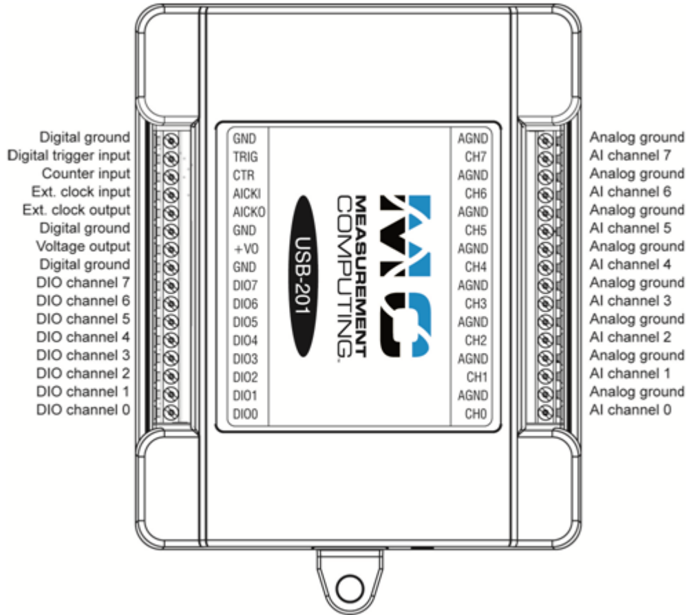
Figure 3. USB-201 pinout
