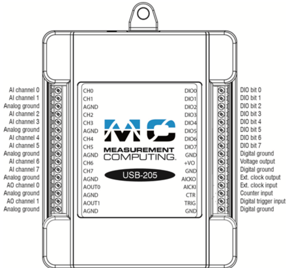
Figure 3. USB-205 pinout
