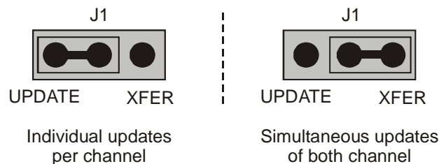
Figure 3. Individual / simultaneous update jumper
