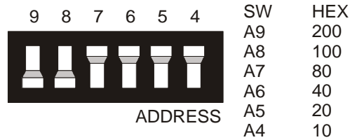
Figure 2. Base address switch
