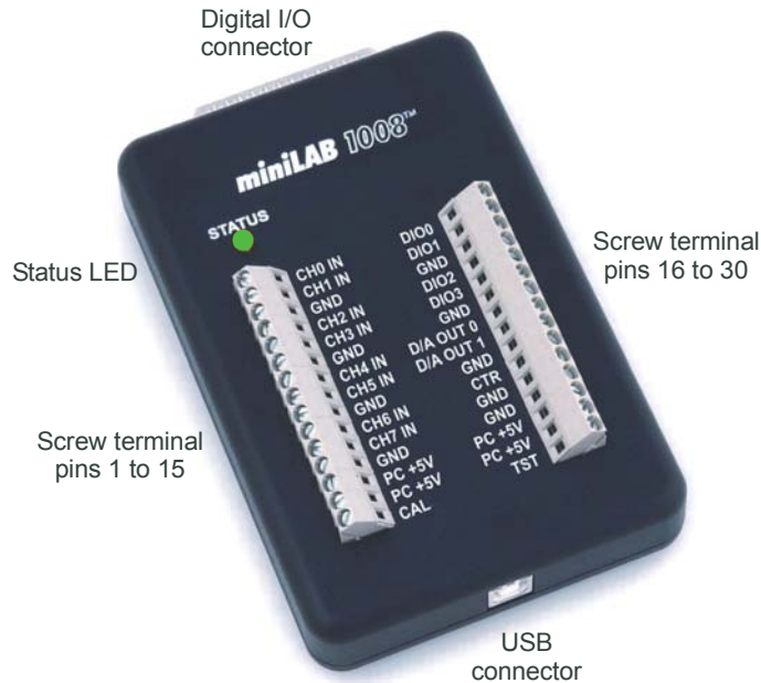
Figure 3-1. miniLAB 1008 external components
