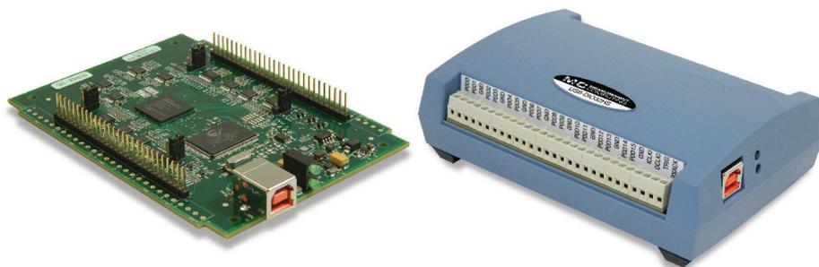
USB-DIO32HS devices provide 32 bits of high-speed digital I/O, input/output scan rates up to 8 MS/s, and simultaneous hardware and software scanning. The USB-DIO32HS-OEM (above left) has a board-only form factor and header connectors. The USB-DIO32HS (above right) is a cased version with screw terminals.
