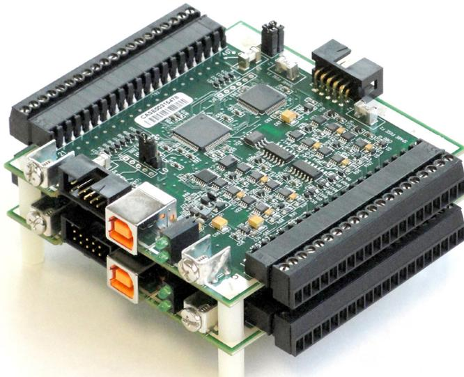
Multiple USB-7000 Series devices can be stacked to increase channel count and capability.
