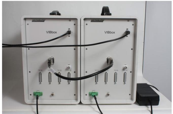
**VIBboxes are connected together by attaching an EP377 Trigger Bus cable from the Sync Bus connector of one VIBbox to the Sync Bus connector of the next VIBbox. Each VIBbox must be powered using an external power supply and connected to a USB 3.0 port of a host computer.**
