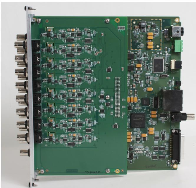
*The DT9857E provides sixteen IEPE analog inputs, 2 analog outputs, 16 DIO, 1 counter/timer, 1 tachometer, and 2 measure counters on each board set. VIBbox-64 packages four of these to bring the channel count to: 64 IEPE analog inputs, 8 analog outputs, 64 DIO, 4 counter/timer, 4 tachometers, and 8 measure counters. For more information on the DT9857E module, visit our web site: [www.mccdaq.com/Products/Sound-Vibration-DAQ/DT9857E](http://www.mccdaq.com/Products/Sound-Vibration-DAQ/DT9857E)*
