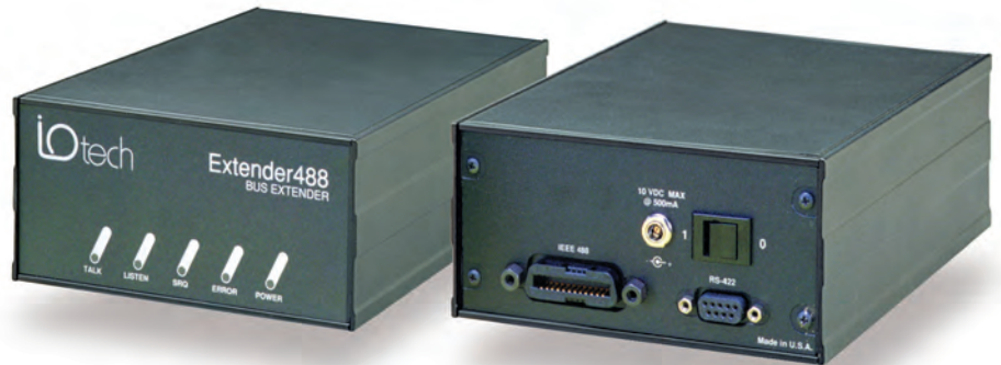
The Extender488 Series enables instruments to be located up to 4,000 feet from host IEEE controller
