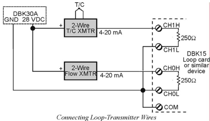
The 28 VDC mode can also be used to provide a 14 VDC excitation source for bridge-type sensors such as load cells (strain gages). The excitation voltage is not regulated by the DBK30A; so, this voltage must be externally regulated to 10.00 V for most load cells.
