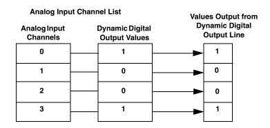
Figure 23: Example Using Dynamic Digital Outputs
