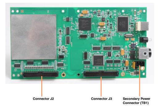
Figure 29: Orientation of Connectors J2 and J3 and TB1
