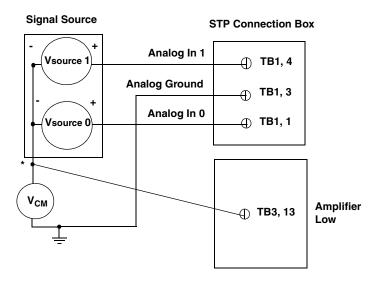
\*Make this connection as close to  $V_{IN}$  sources as possible to reduce ground loop errors.  $V_{cm}$  is the common mode voltage for all analog inputs.
