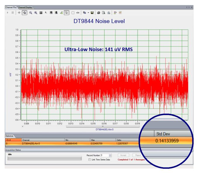
Figure 27 shows the typical system noise of the DT9844 module. (QuickDAQ was used to acquire and display the data.)
