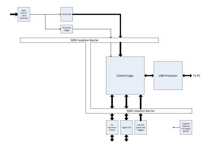
Figure 22 shows a block diagram of the DT9844 module.
