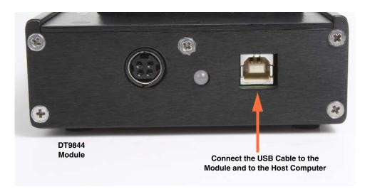
Figure 4: Attaching the Module to the Host Computer
