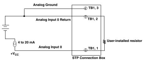
The user-installed resistor connects the high side of the channel to the low side of the corresponding channel, thereby acting as a shunt. For example, if you add a 250  $\Omega$  resistor and then connect a 4 to 20 mA current loop input to channel 0, the input range is converted to 1 to 5 V.
