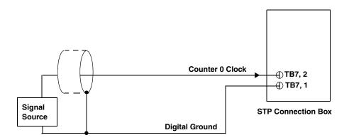
Figure 18: Connecting Counter/Timer Signals to the STP Connection Box for a Period/Pulse Width Measurement Operation
