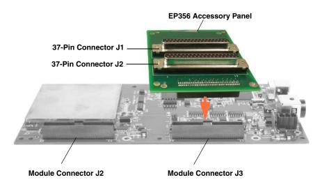
Figure 34: Connecting the EP356 Panel to the DT9844-32-OEM Module
