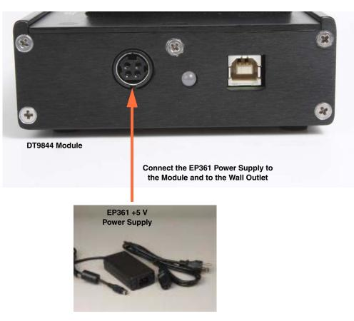
Figure 3: Attaching a +5 V Power Supply to the DT9844 Module
