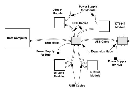
Figure 5: Attaching Multiple DT9844 Modules Using Expansion Hubs
