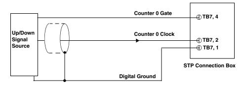
Figure 16: Connecting Counter/Timer Signals to the STP Connection Box for an Up/Down Counting Operation
