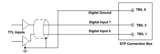
Figure 12: Connecting Digital Inputs to the STP Connection Box
