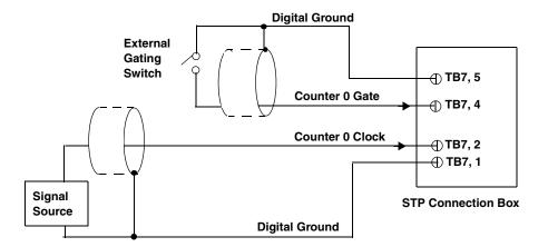
Figure 14: Connecting Counter/Timer Signals to the STP Connection Box for an Event Counting Operation Using an External Gate
