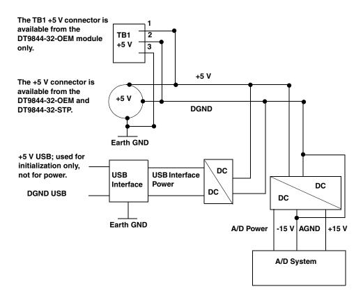
Figure 40: Ground, Power, and Isolation Connections
