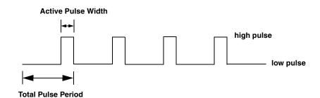
Figure 26: Example of a Low-to-High Pulse Output Type
