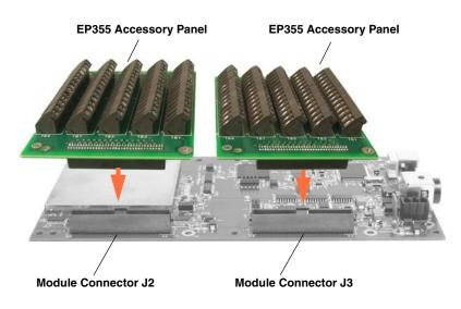
Figure 38: Connecting the EP355 Panel to the DT9844-32-OEM Module
