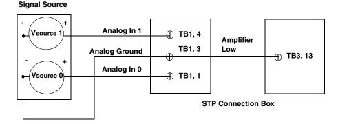
Figure 7: Connecting Single-Ended Inputs to the STP Connection Box
