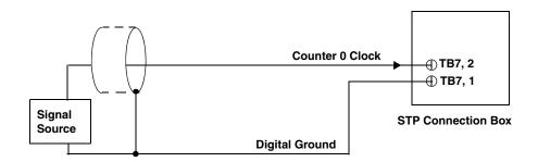
Figure 15: Connecting Counter/Timer Signals to the STP Connection Box for an Event Counting Operation Without Using a Gate
