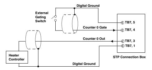
Figure 21: Connecting Counter/Timer Signals to the STP Connection Box for a Pulse Output Operation Using an External Gate
