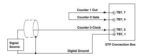
Figure 17: Connecting Counter/Timer Signals to the STP Connection Box for a Frequency Measurement Operation Using an External Pulse
