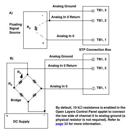
Figure 9: Connecting Differential Inputs to a Screw Terminal Panel
