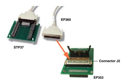
Figure 33: Connecting the STP37 Screw Terminal Panel to Connector J2 of the EP353 Accessory Panel Using the EP360 Cable
