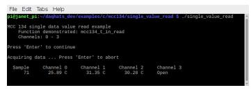
Continuously read and display the value of each thermocouple input
