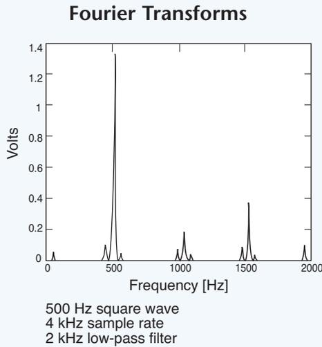
**Fig. 3.09.** The Fourier Transform of a 500 Hz square wave is sampled at 4 kHz with a low-pass filter cutoff at 2 kHz.
