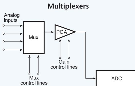
**Fig. 3.01.** The multiplexer (MUX) is a fast switch that sequentially scans numerous input-signal channels and directs them in a preprogrammed manner to a single ADC for digitizing. This approach saves the cost of using an ADC for each channel.
