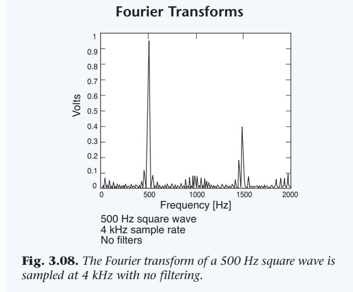
**Fig. 3.08.** The Fourier transform of a 500 Hz square wave is sampled at 4 kHz with no filtering.
