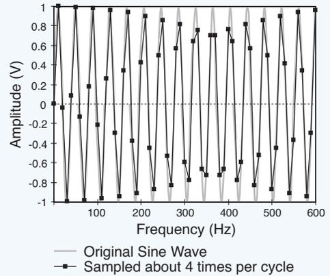
**Fig. 3.07.** When ac inputs are sampled more than twice the Nyquist frequency of the sine wave, the frequency content of the signal is preserved, and all the Fourier components of the periodic waveform are recovered.
