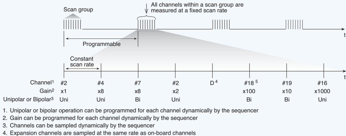
**Fig. 3.02.** This is an example of a 512 location scan sequencer operating in a 100 kHz data acquisition system. The sequencer can program each channel dynamically for unipolar or bipolar operation. The sequencer also can program the gain for each channel on the fly and change the order in which the channels are scanned.
