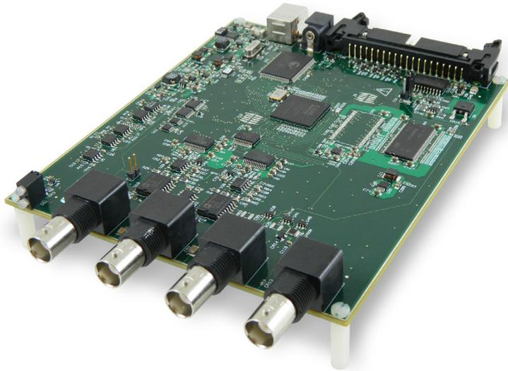
The USB-2020 offers high-speed simultaneous sampling at rates up to 20 MS/s per channel to onboard memory.
