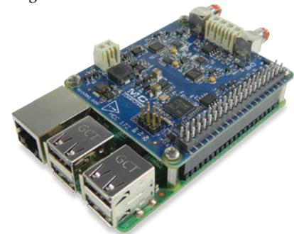
*The MCC 172 is an IEPE measurement DAQ HAT for Raspberry Pi with 2 simultaneous inputs, 24-bit resolution, 51.2 kS/s/ch sample rate and 1 digital input.*
