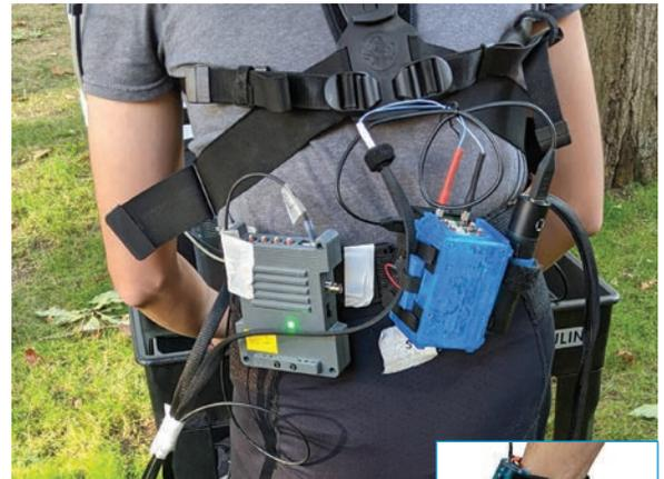
*The small size of the Raspberry Pi and MCC 172 allowed researchers to create a lightweight and wearable DAQ solution to measure dynamic activity during walking and running.*
