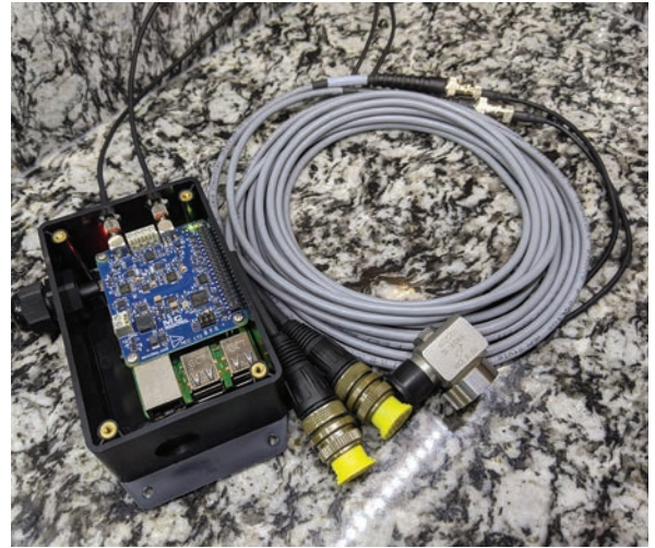
The MCC DAQ HATs fit easily within the existing system enclosure.
