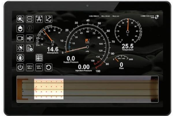
*Data is sent via WiFi to a remote touch screen interface where the operator can view gas pressure, temperature, and flow data in real time.*
