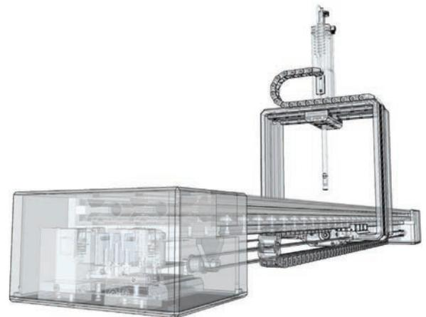
*The Probe Permeameter machine makes measurements in core samples using an X-Y control system with under one millimeter precision. A Raspberry Pi 4 board is at the heart of the solution, providing enough processing power for the machine vision and data acquisition and control functions.*
