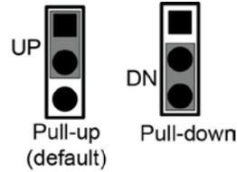
Figure 6. Pull-up/down jumper configurations, typical
