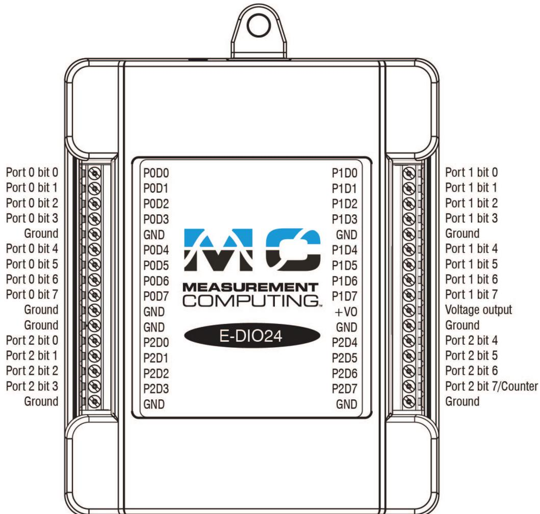
Figure 2. E-DIO24 pinout
