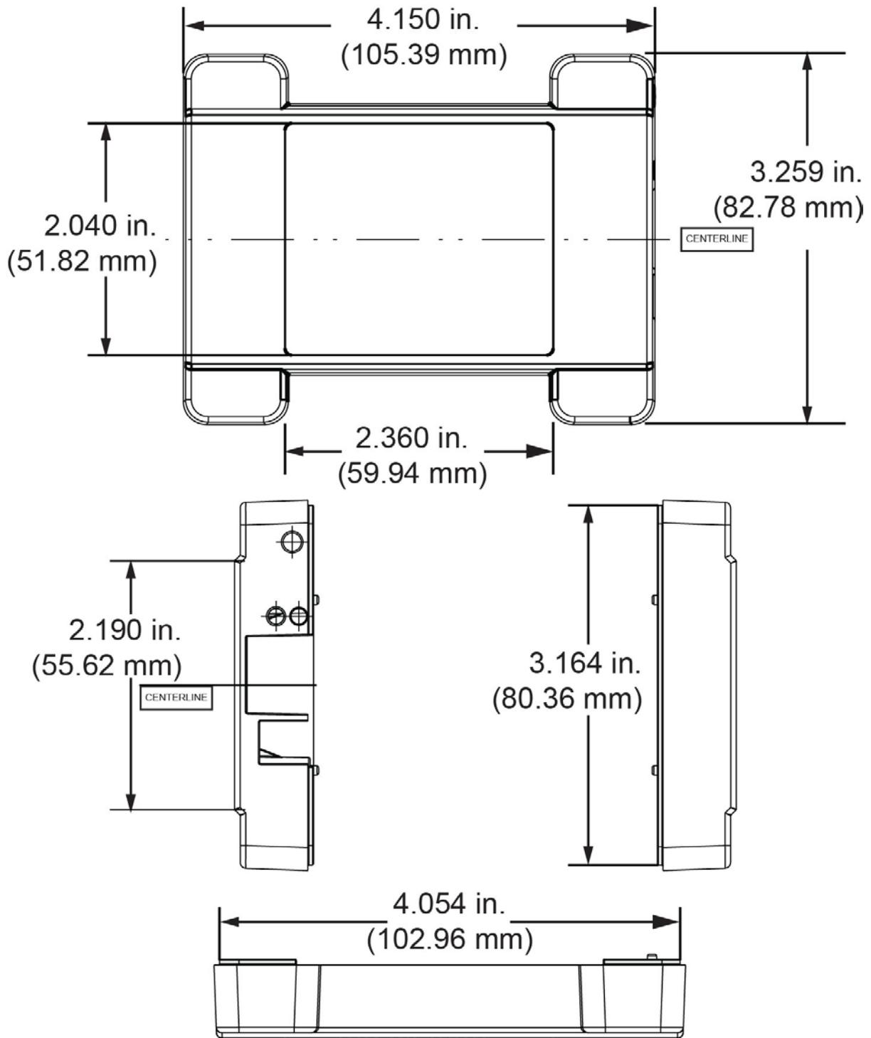
Figure 9. E-DIO24 top enclosure dimensions
