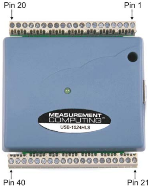
Figure 3-2. USB-1024HLS screw terminal pin numbers
