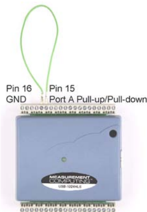
Figure 3-6. Pull-down connection for Port A
