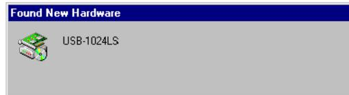
Another **Found New Hardware** balloon or dialog opens after the first closes that identifies the USB-1024LS as a USB Human Interface Device. This balloon or dialog indicates that your USB-1024LS is installed and ready to use.
