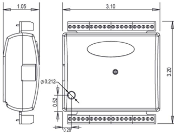
Figure 15. Circuit board (top) and enclosure dimensions
