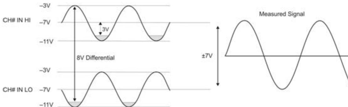
Figure 7. Differential voltage example: common mode voltage of -7 V
