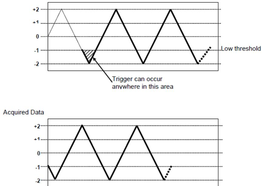
Figure 12. Trigger below, level-sensitive
