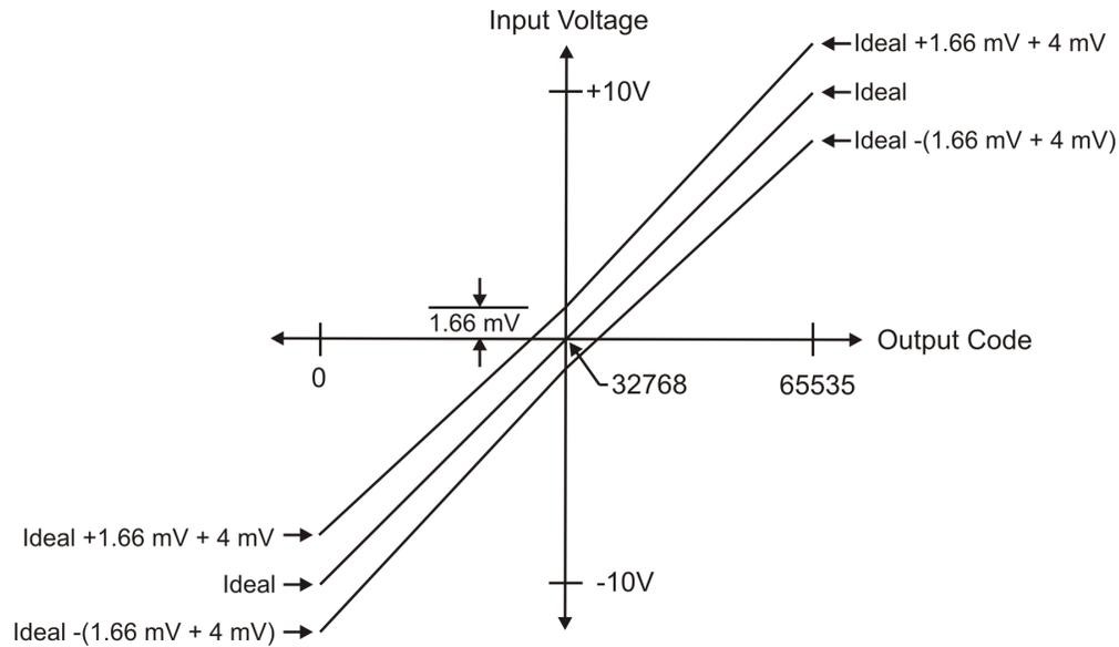
Figure 8. USB-1616FS error band plot
