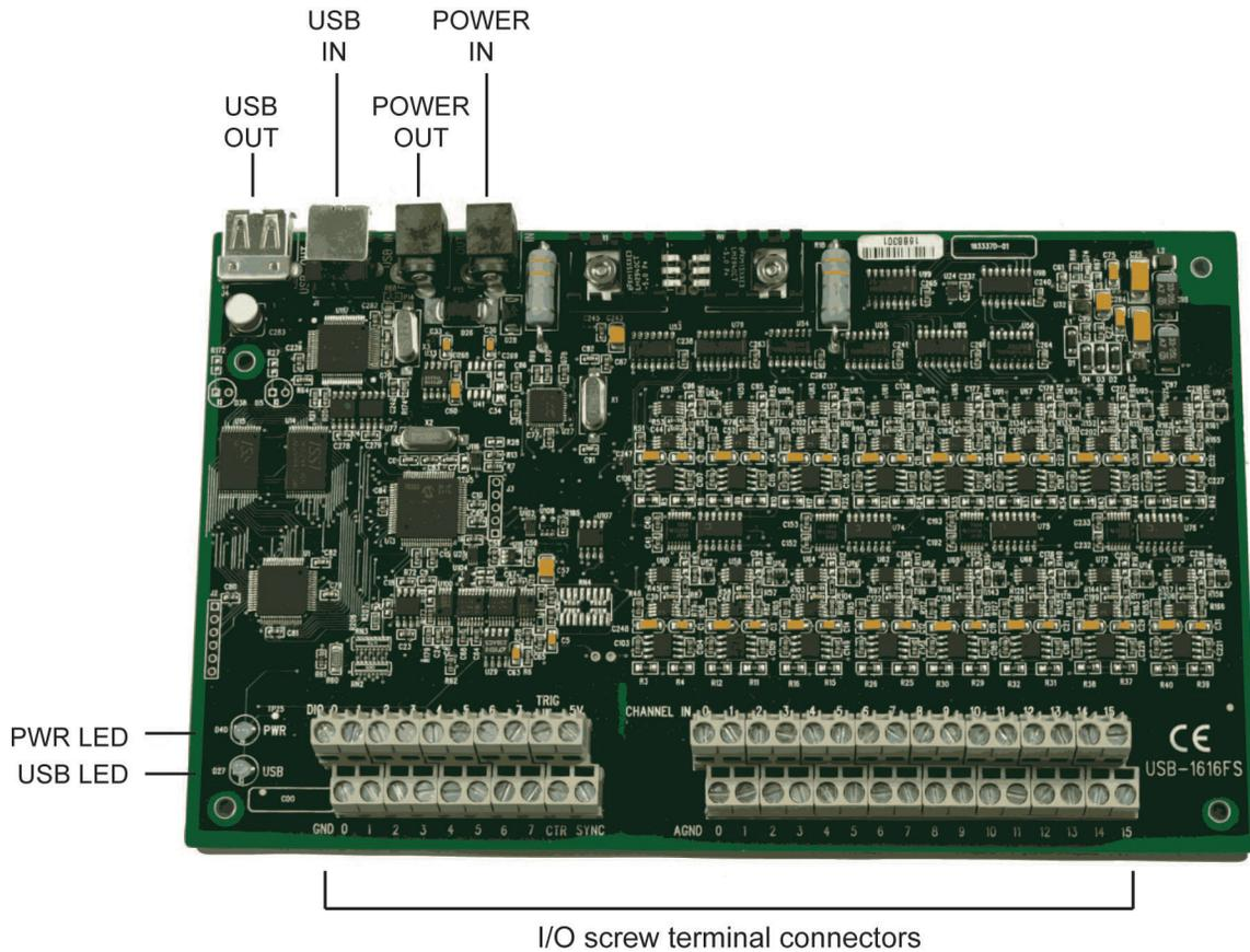
Figure 2. USB-1616FS internal components
