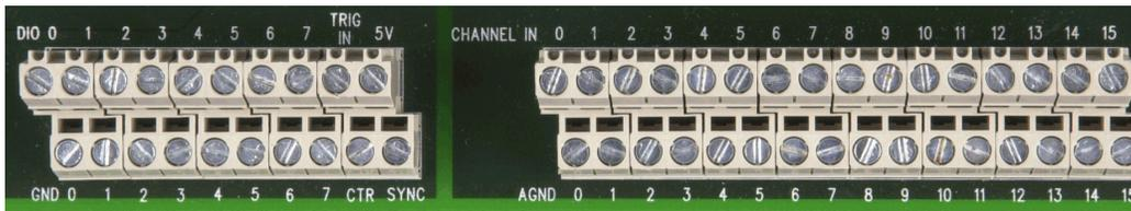
Figure 3. USB-1616FS screw terminals
