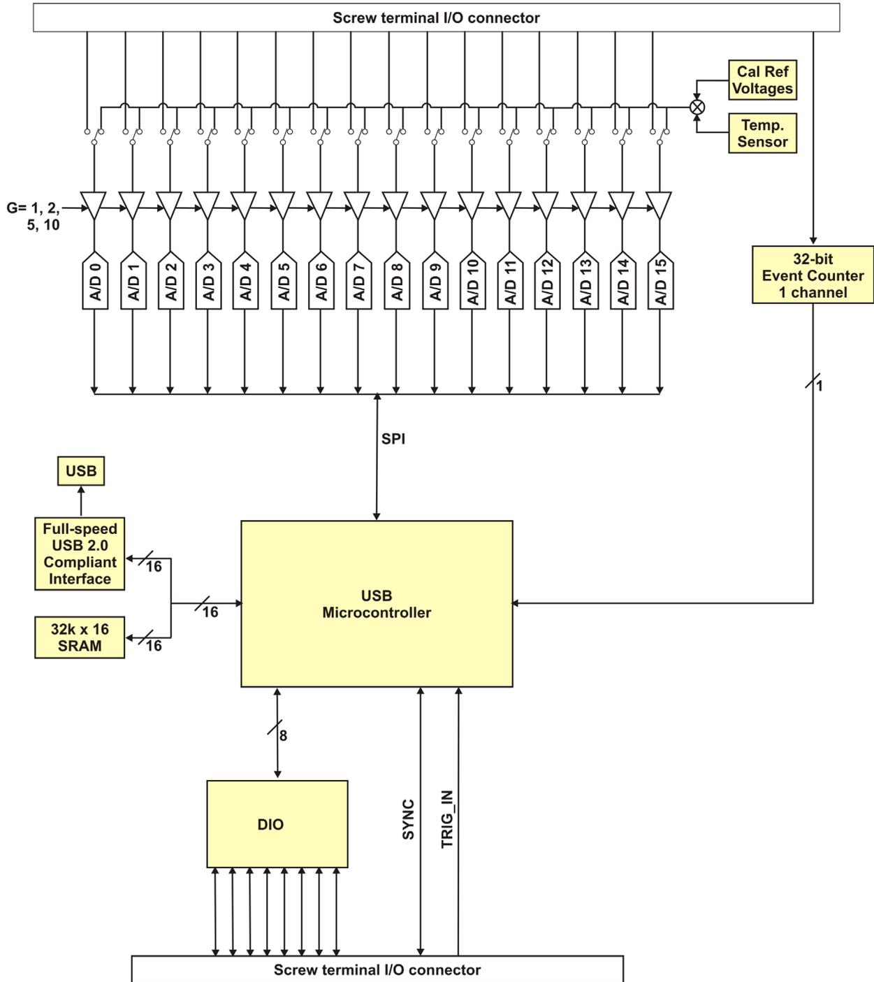
Figure 1. USB-1616FS functional block diagram
