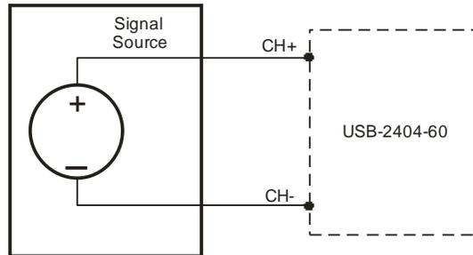
Figure 6. Connecting a floating signal source
