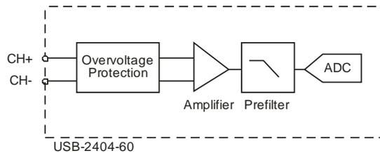
Figure 7. Analog input circuitry for one channel
