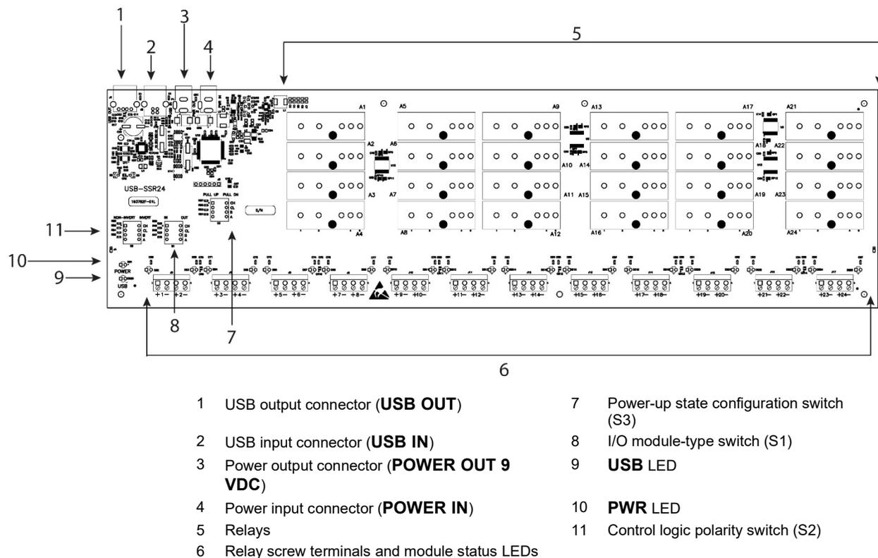
Figure 6. USB-SSR24 components
