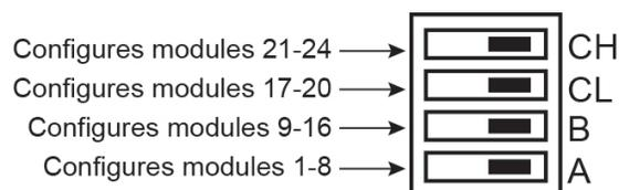
Figure 2. Typical PCB switch
