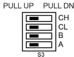
Figure 9. Switch S3 default configuration
