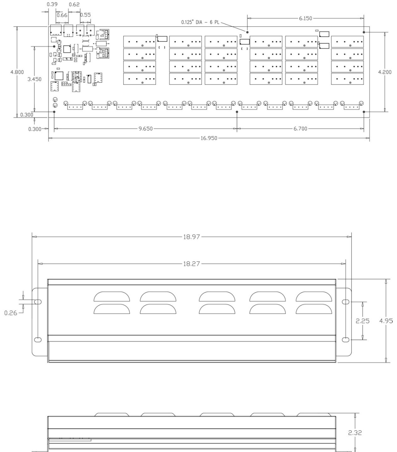
Figure 11. Circuit board (top) and housing dimensions
