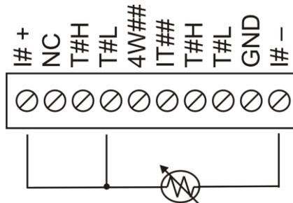
Figure 6. Three-wire RTD or thermistor sensor measurement configuration
