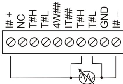
Figure 8. Four-wire, single RTD or thermistor sensor measurement configuration
