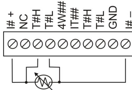
Figure 7. Four-wire, single RTD or thermistor sensor measurement configuration
