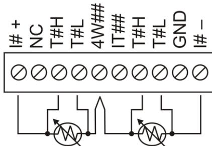
Figure 9. Four-wire, two RTD or thermistor sensors measurement configuration
