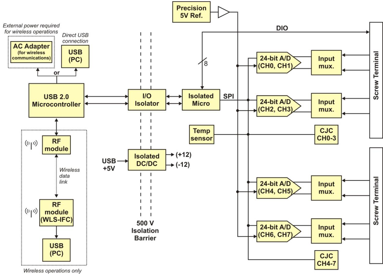
Figure 1. WLS-TC functional block diagram
