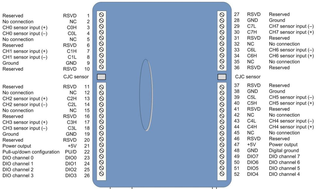
Figure 2. WLS-TC screw terminal pin numbers
