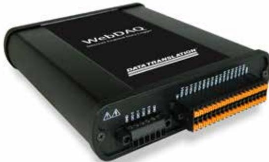
The WebDAQ DT5828 intelligent logger features remote monitoring and control of real-time temperature data.
