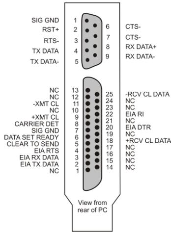
The **CIO-COM422** combines an RS232 and an RS422 interface with a single communications port. RS232 is commonly a 25-pin connector, while RS422 is a 9-pin connector.
