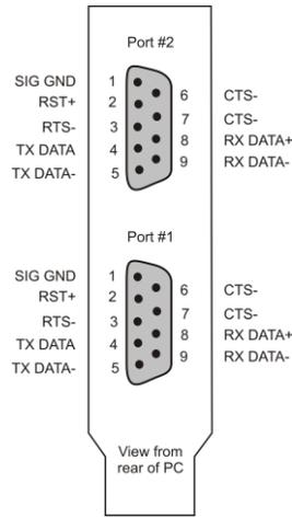
The **CIO-DUAL422** combines a pair of communications ports each with RS422 standard interfaces. Each COM port uses one of the 9-pin connectors shown here.
