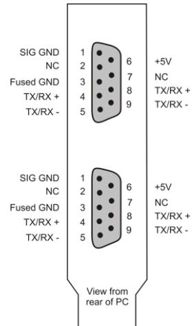
The **CIO-COM485** is equipped with two DB9 connectors for RS485 standard 9-pin connectors and cables. The RS485 standard allows multiple transmitters and receivers on a single communications cable.
