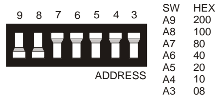
Figure 2. Base address switches (300h shown)
