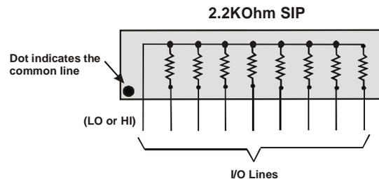
Figure 6. Eight-resistor SIP schematic
