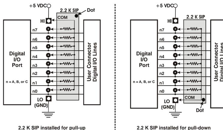
Figure 7. Pull-up and pull-down resistor SIPs schematic
