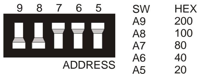
Figure 1. Base address switch
