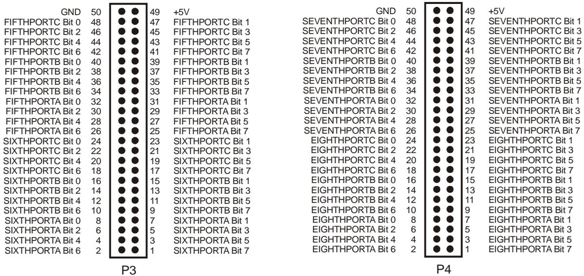
Figure 4. P3 and P4 pin out
