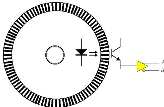
The concentric pattern for B has the same number of window pairs as A except that the entire pattern is rotated by 1/4 of a window-pair. Thus the B signal will always be 90 degrees out of phase from the A signal. The A and B signals will pulse 512 times (or 1024, 4096, etc.) per complete rotation of the encoder.
