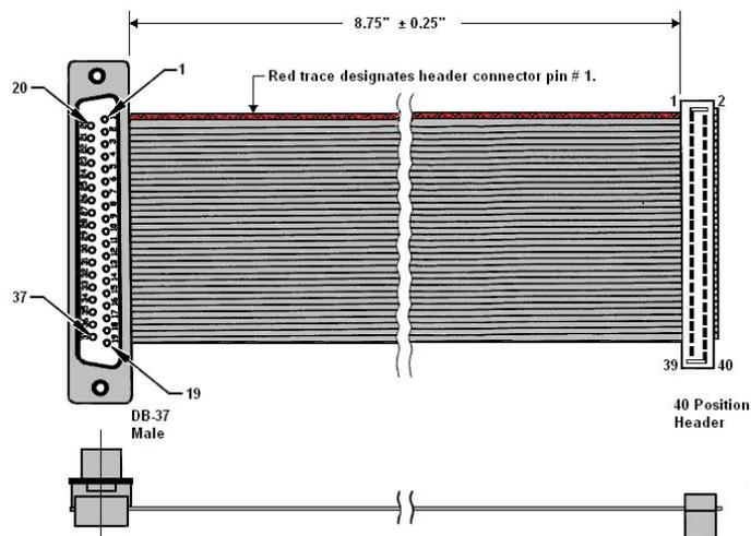
**CA-248 Pinout, DB-37 Pins listed Sequentially**
