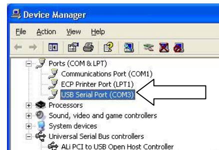
Figure 5. USB Serial Port (COM) The desired result.
