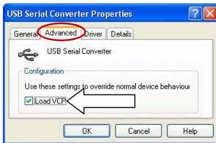
Figure 4. Checking “Load VCP” in the Advanced Tab
