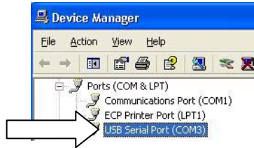
Figure 1. The USB Serial Port (Correct)
