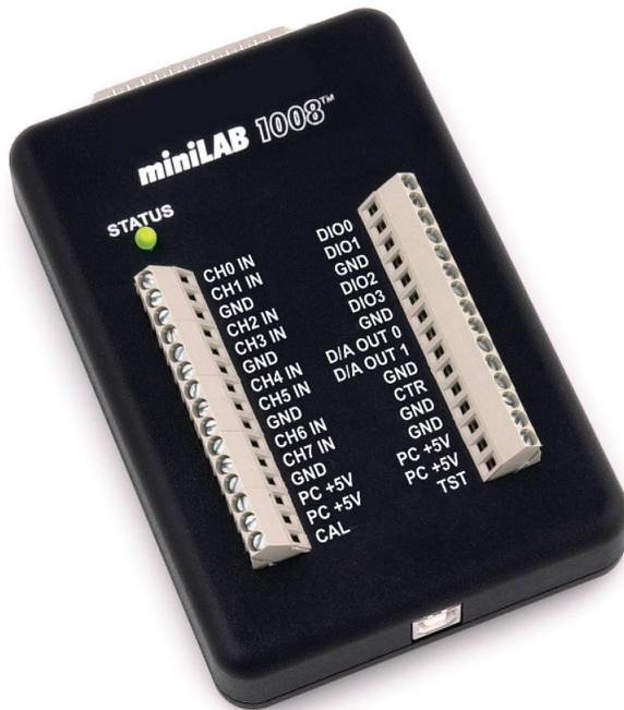
The miniLAB 1008 features 8 single-ended or 4 differential analog inputs, two analog outputs, 28 bidirectional DIO lines, one 32-bit event counter, and a rugged enclosure
