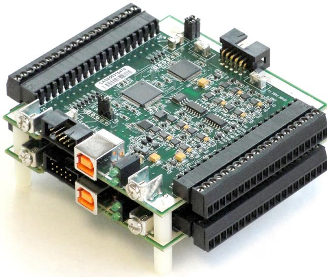
Multiple USB-7000 Series devices can be stacked to increase channel count and capability.
