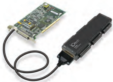
DaqBoard/3000 attached to a PDQ30 expansion module
