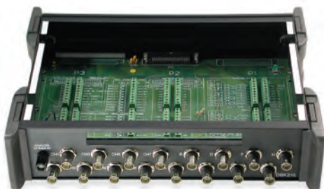
DBK215 shown with cover removed, providing access to all screw terminals
