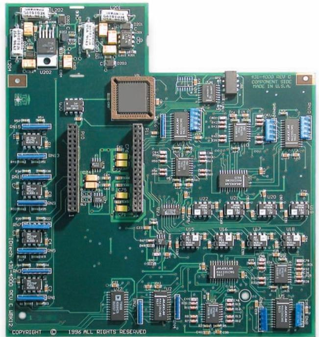
WBK12A and WBK13A are 8-channel programmable low-pass filter cards for use with WaveBook data acquisition systems. These cards, which install\* directly into any WaveBook system or WBK10A expansion module, provide programmable low-pass filtering over all channels. The WBK13A further enables the simultaneous sampling of all channels\*\*. If simultaneous sample and hold is installed in multiple modules, then all channels are sampled within 100 ns of one another.
