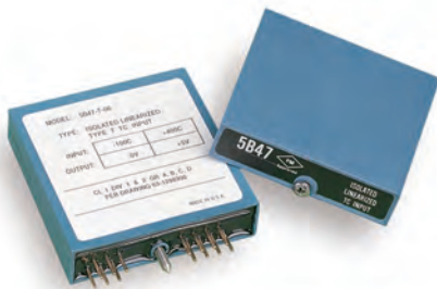
5B modules selected from a choice of types are placed into the WBK15 module
